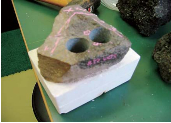
Fig. 2 Plaster-immobilized specimen (left photo) and trimmed specimens for measurement (right photo). The larger cylindrical specimen in the photo on the right is for measurement of magnetization, while the smaller for measurement of susceptibility.
