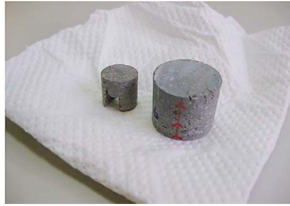
Fig. 2 Plaster-immobilized specimen (left photo) and trimmed specimens for measurement (right photo). The larger cylindrical specimen in the photo on the right is for measurement of magnetization, while the smaller for measurement of susceptibility.
