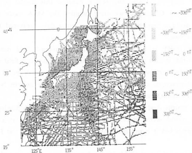
Fig. 4. A magnetic anomaly chart of maritime geomagnetic total intensity observed in 1961–1979 based on the IGRF model. [A reproduction of Fig. 2 of Fujita and Kawamura (1984)].
